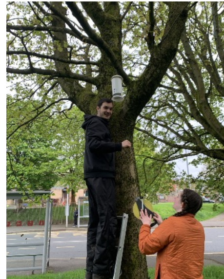
Figure 2. GALLANT team setting up a temperature/humidity logger with radiation shield
