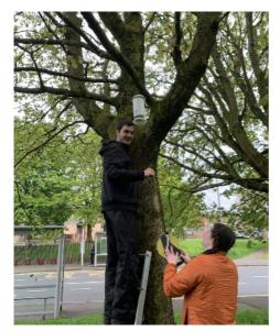
Figure 2. GALLANT team setting up a temperature/humidity logger with radiation shield
